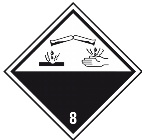
Corrosive hazard label
