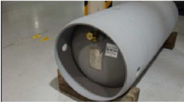
Figure 5: Type 30B Cylinder
