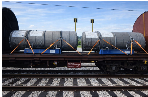
Figure 10: 48Y Cylinder on with BTP outer protection
