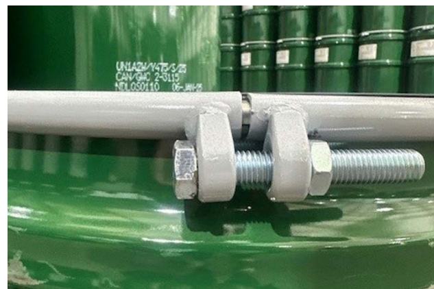
Image 3.4b Standard drum lid with C or U section locking ring
