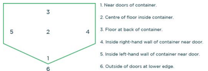
Image 11a - Six Minimum Prescribed Locations in an ISO shipping Container
