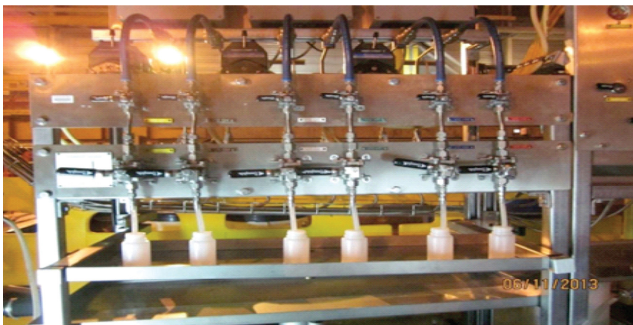
Figure 4: The manual sampling rigs extracts the liquor from the trial containers and sent to the site laboratories for analysis for Cs137, nickel and cobalt.
