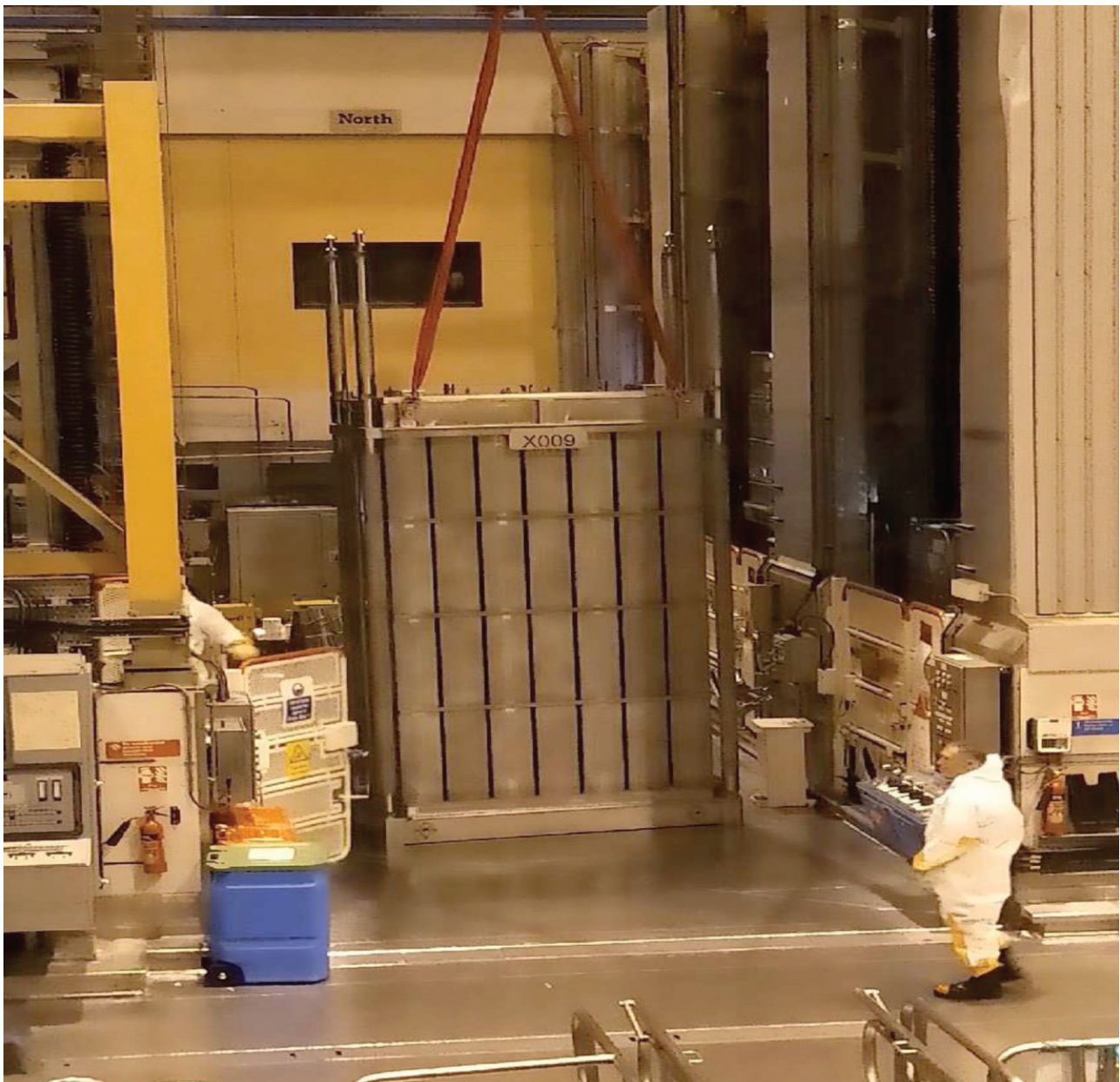
Figure 10: This is the most recent picture of a 63c rack being imported into TR&S preparation area, on completion of quality checks it will be transported to the pond for fuel handling trials.
