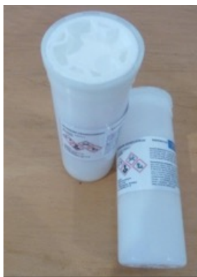
Plastic pot (inner packaging for liquid dangerous goods in combination packaging) with large opening as secondary packaging with GHS markings
