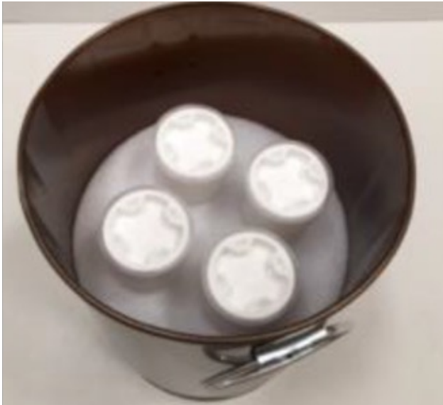
4 secondary packagings wrapped in a UN 1A2/X steel drum
