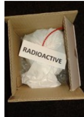
Secondary packaging wrapped in the outer packaging with the mark "RADIOACTIVE"
