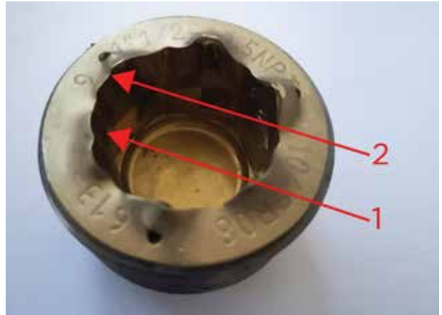
Figure 3: Example of an unacceptable deformation of the socket caused by tool bit which was not fully inserted during installation (1). One can see that the tool has been withdrawn during the installation (2).
