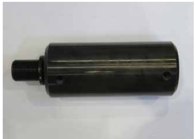
Figures 5 a/b: Example of a hardened 1" tool bit with its hardened holder
