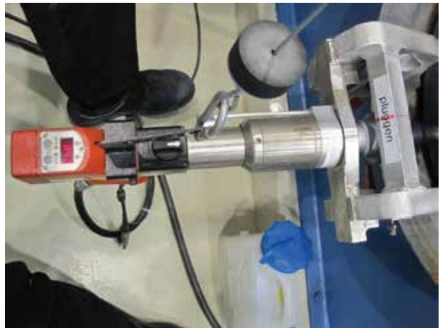
Figure 11: Example of a torque reaction hanging bracket (general view)
