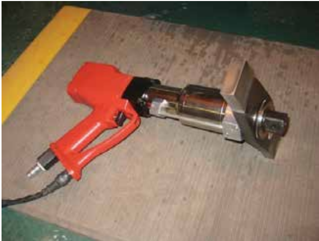
Figure 8: Example of a torque device with a double reaction arm
