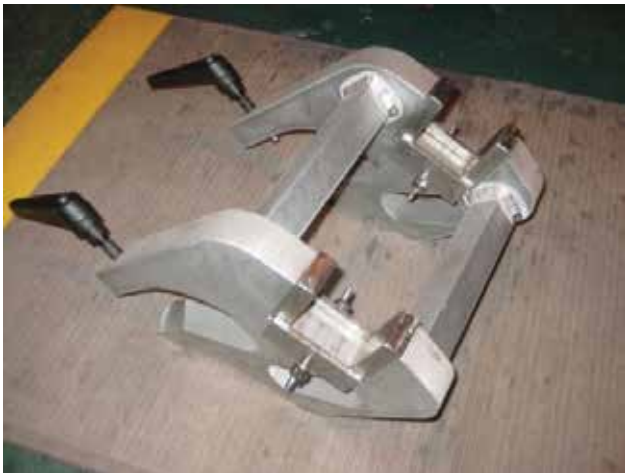
Figure 9: Example of a torque reaction hanging bracket
