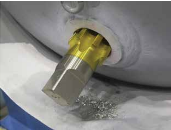
Figure 2: Tap inserted into a cylinder coupling (paper has been moistened with alcohol to attract loose particles, but this is not required)
