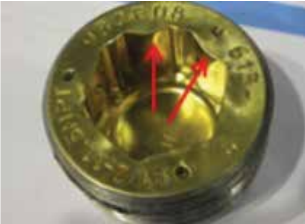
Figure 1: Example of an unacceptable deformation of the socket caused by too large of a gap between the tool bit and the socket
