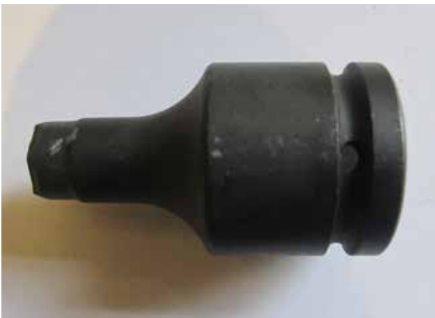
Figure 2: Broken 1" tool bit
