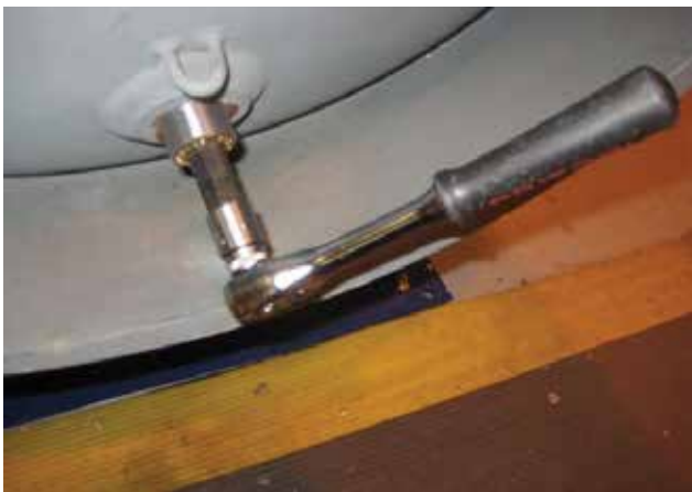
Figure 29: Example of insertion of a socket head plug with ratchet spanner till tight
