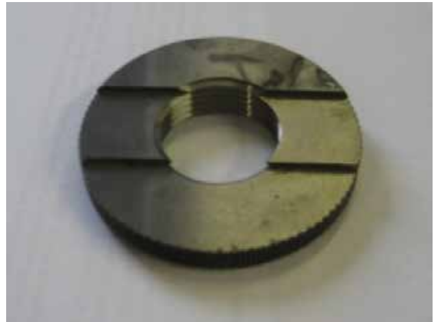
Figure 5: Example of a standard NPT gauge
