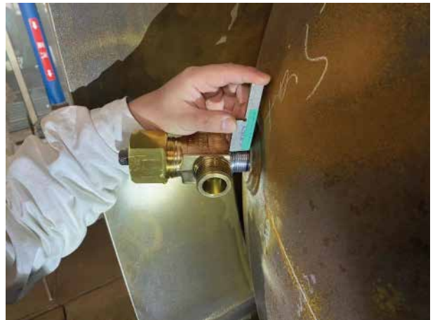
Figure 27: "no-go" side of gauge must not fit
