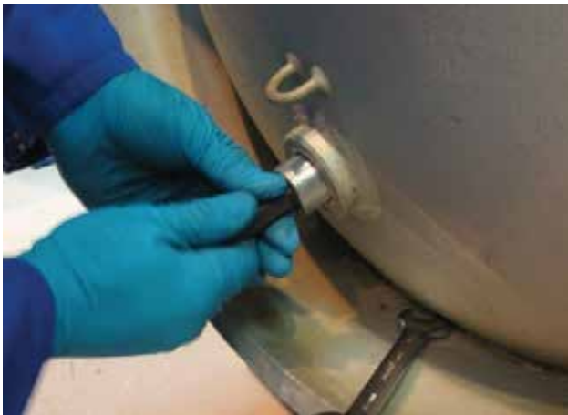
Figure 28: Example of insertion of a socket head plug by hand
