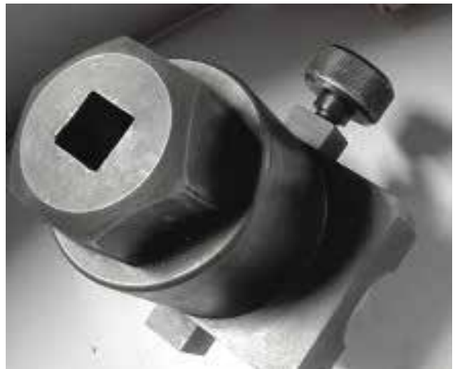
Figure 15: Example of a complete assembled special adapter for the valve
