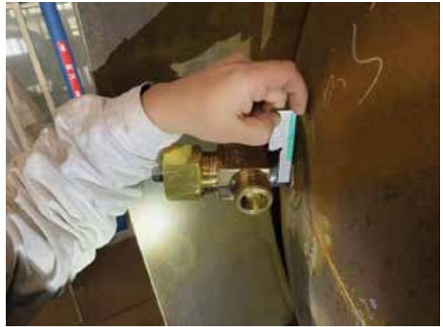
Figure 26: "go" side of gauge must fit
