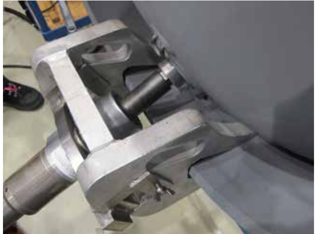
Figure 10: Example of a torque reaction bracket between the tool and the skirt
