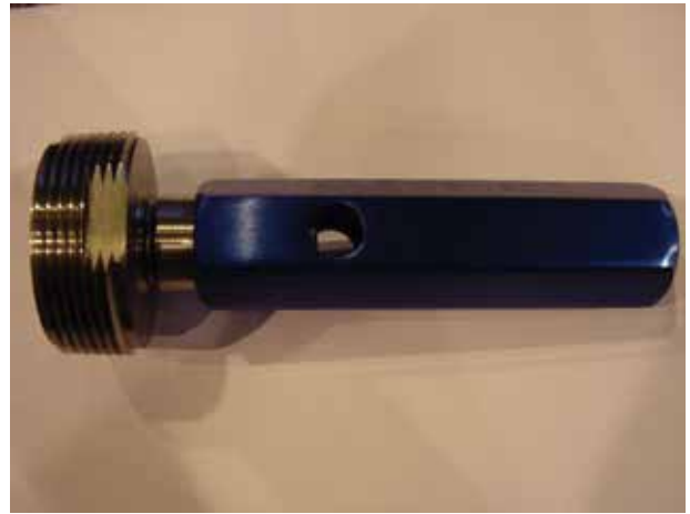
Figure 3: Example of a standard NPT gauge
