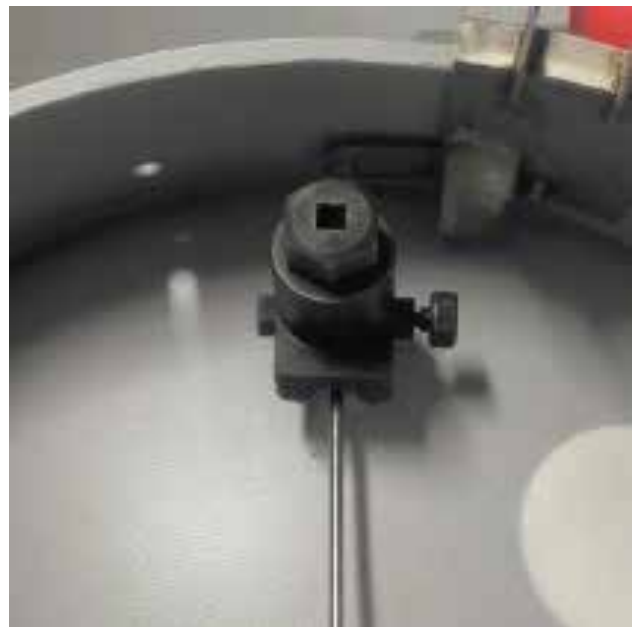
Figure 16: Example of a special tool for positioning valve, the pin is installed in the outlet port of the valve
