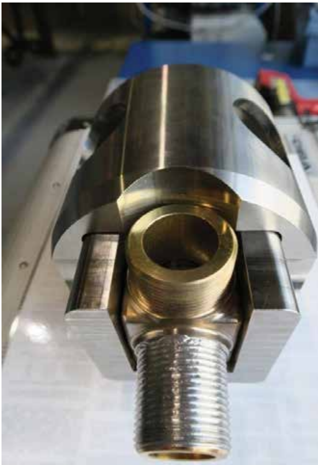
Figure 14: Example of a special tool to fully cover the valve body with minimum clearance between the valve body and the tool
