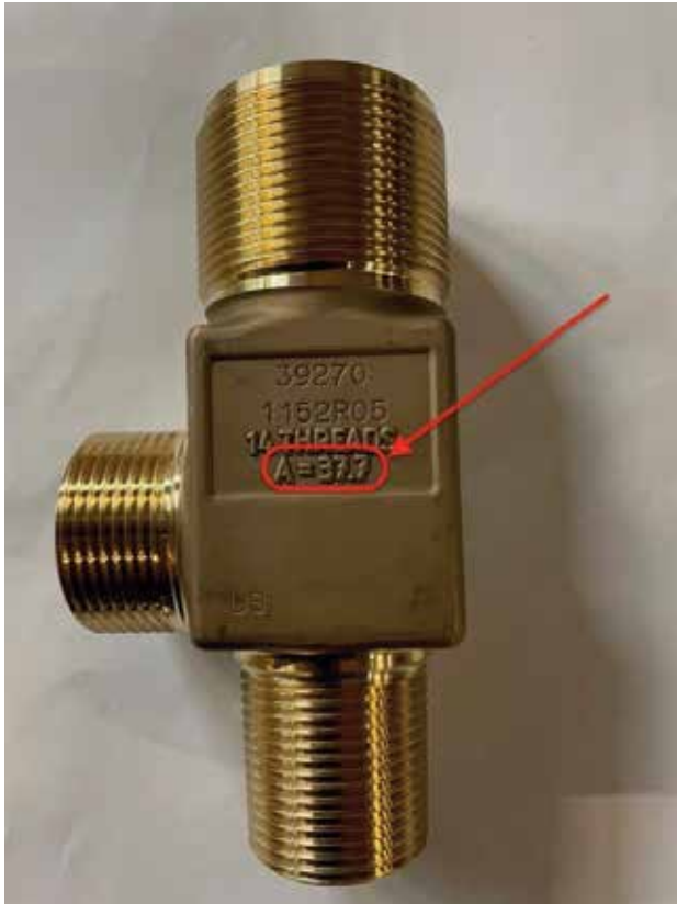
Figure 23: Reference dimension A stamped on valve body
