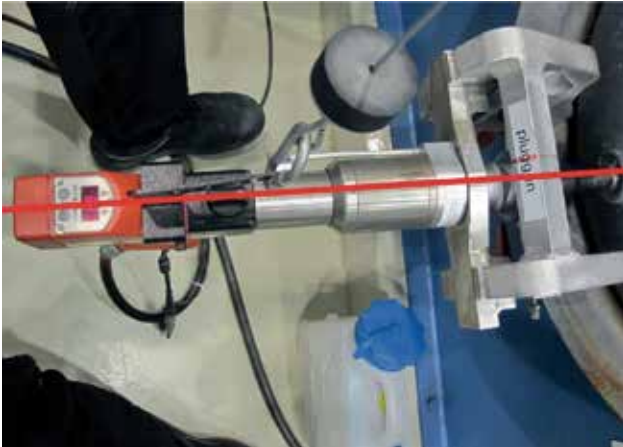
Figure 31: Example engaging the tool bit within the center of a socket head plug
