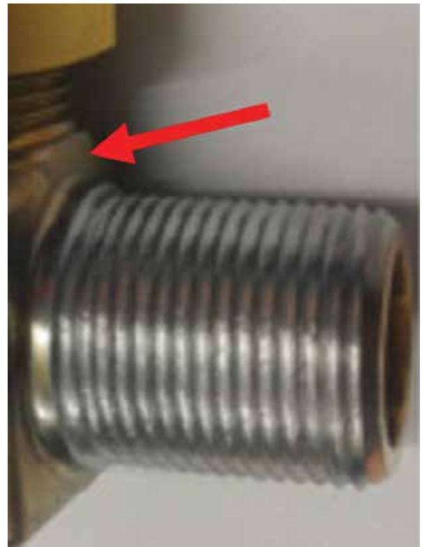
Figure 24: Machined reference surface on a valve
