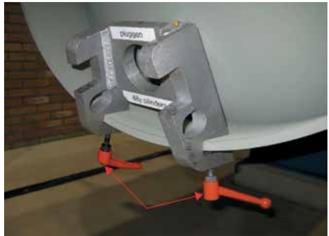
Figure 30: The torque reaction hanging bracket and locking screws
