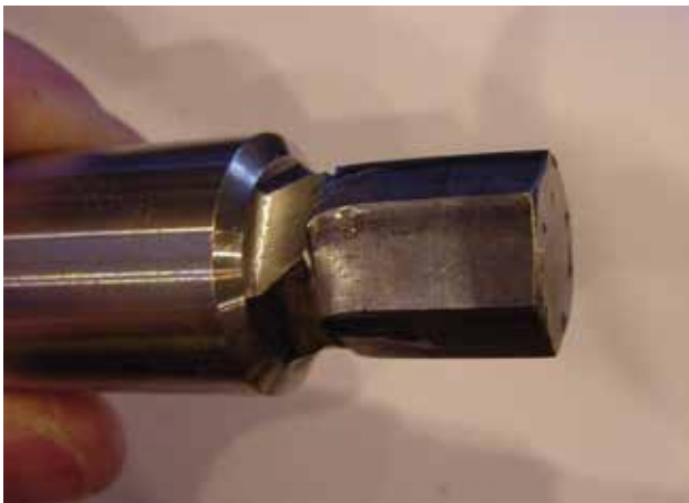
Figure 1: Distorted 1" tool bit
