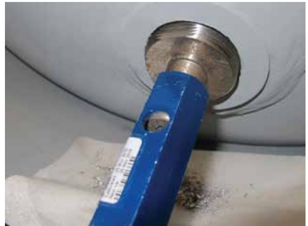
Figure 4: NPT gauge inserted into a cylinder coupling
