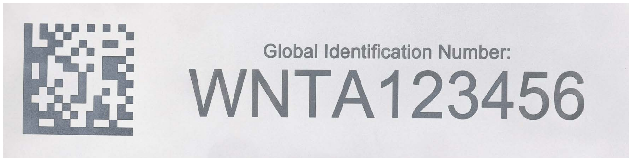
Figure 3. Example global identifier containing 10-character global identification number with 2D barcode
