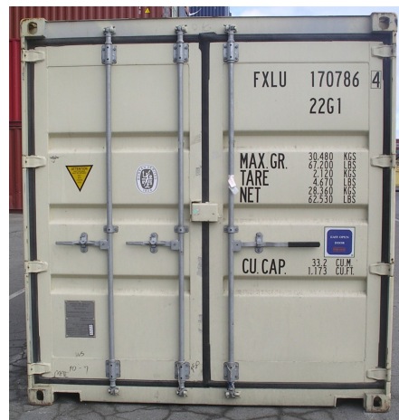
Figure 4a A rare example of a container with three door locking mechanisms
