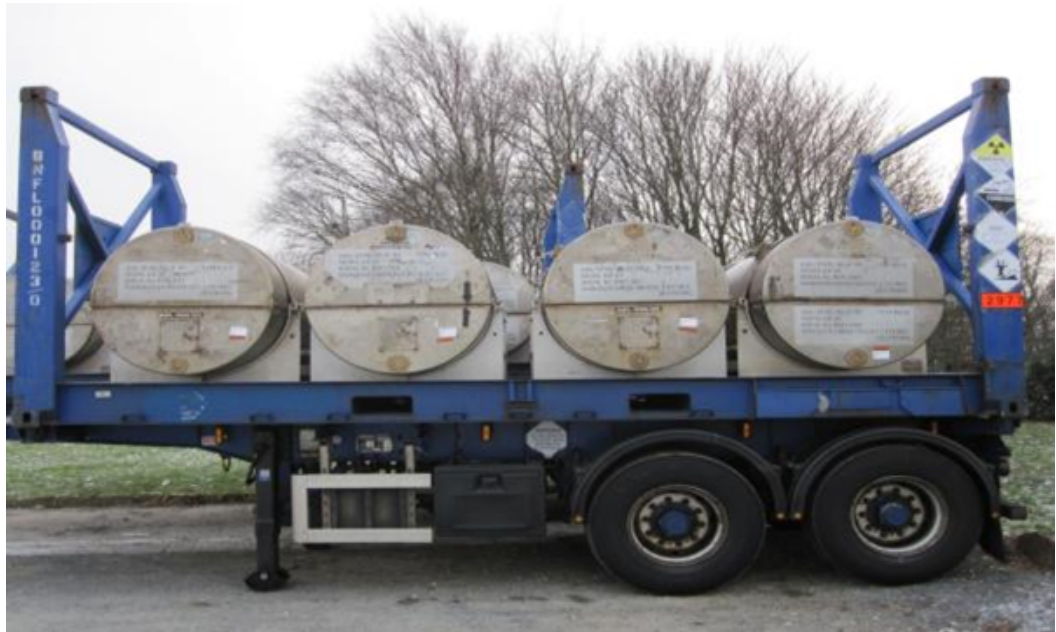
Fig (1) 20FT Fixed Post Flatrack (30B cylinder packed in type UX-30 outer packagings)
