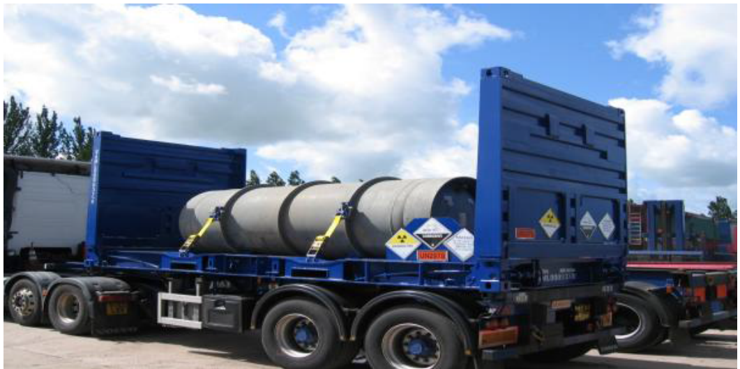
Fig (2) 20FT Flatrack loaded with a 48Y package (with no thermal protection)
