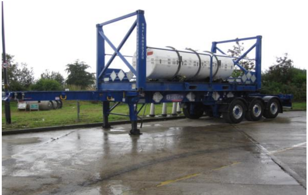
Fig (3) 20FT Fixed Post Flatrack with a 48Y package (with Composite Thermal Protector)
