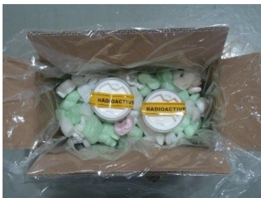
2 secondary packagings wrapped in a UN 4/GV/X fibreboard box as outer packaging with the mark “RADIOACTIVE”
