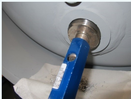
Figure 3: NPT gauge inserted into a cylinder coupling
