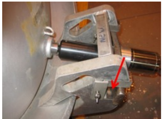
Figure 13: Clearance between the double sided torque reaction arm and the torque reaction hanging bracket.
