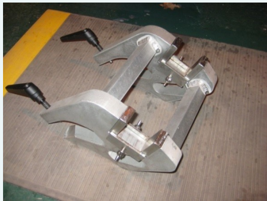
Figures 6 a / b: Example of torque device with a double sided torque reaction arm and torque reaction hanging bracket.
