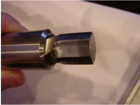
Figure 8 a / b: Distorted and broken tool bits
