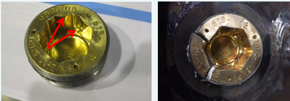
Figure 7 a / b: Example of unacceptable deformation and a cracked plug
