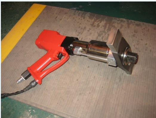
Figures 6 a / b: Example of torque device with a double sided torque reaction arm and torque reaction hanging bracket.
