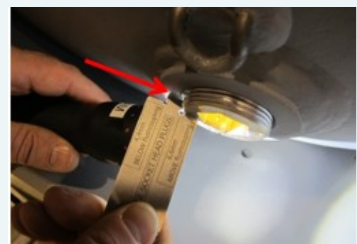
Figure 15: URENCO gauge (+6.6mm side is showing). Note a gap is showing between the outer surface of coupling and the gauge and therefore the plug installation is not sufficient.
