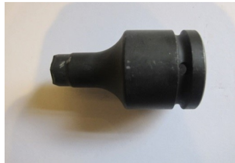
Figure 8 a / b: Distorted and broken tool bits
