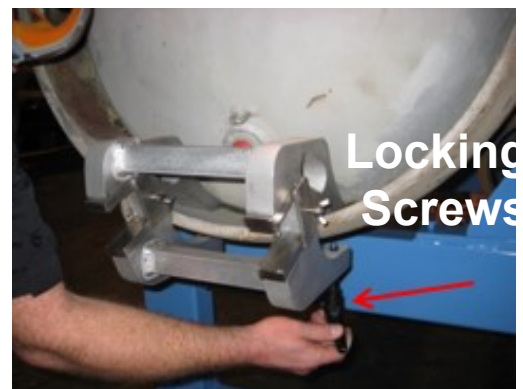
Figure 11: The torque reaction hanging bracket and locking screws.
