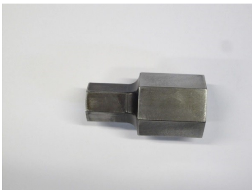
Figure 9 c / d Example of hardened tool bit and adapter
