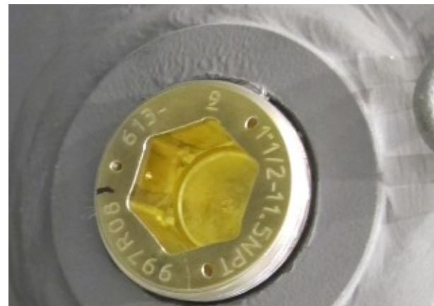
Figures 16 a / b: Examples of acceptable deformation
