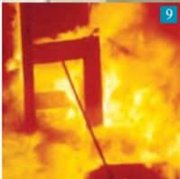
is subjected to a fully engulfing fire of 800°C for 30 minutes;
