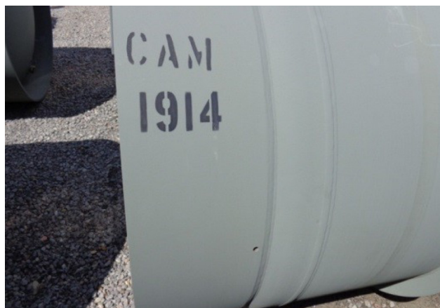
Figure B-2. Cylinder owner applied stencil.
