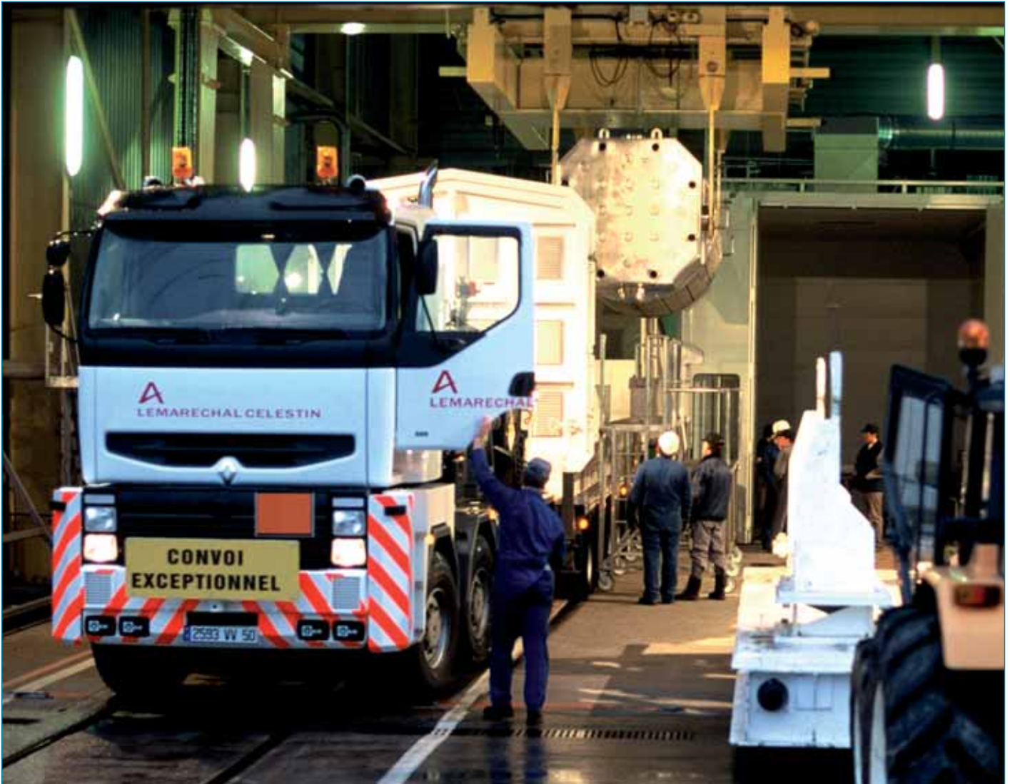
above: Off-loading spent fuel cask for radiological inspection
